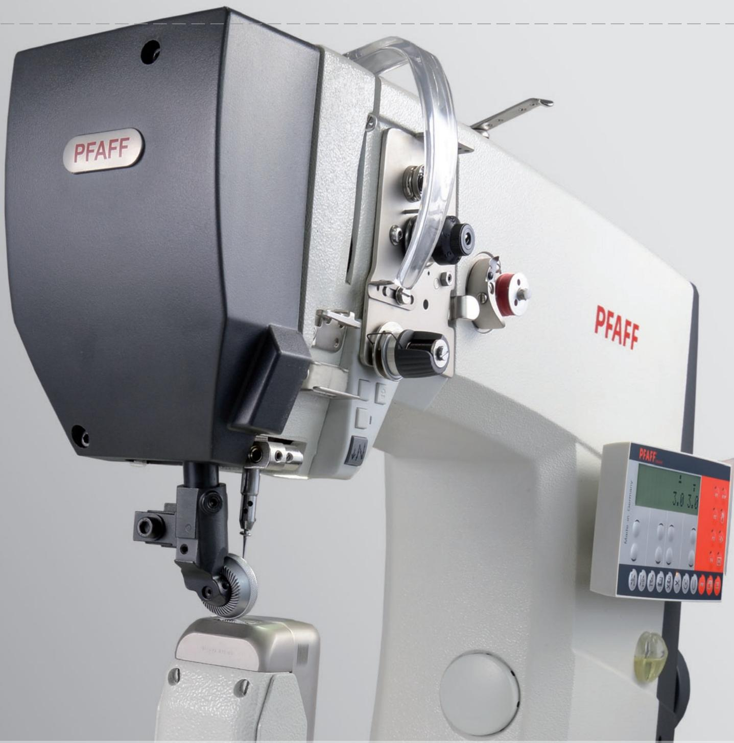
Hot key (forward/reverse) and 3 further keys for the most important adjustment possibilities in the reaching area of the operators hands. Integrated LED-Light.
